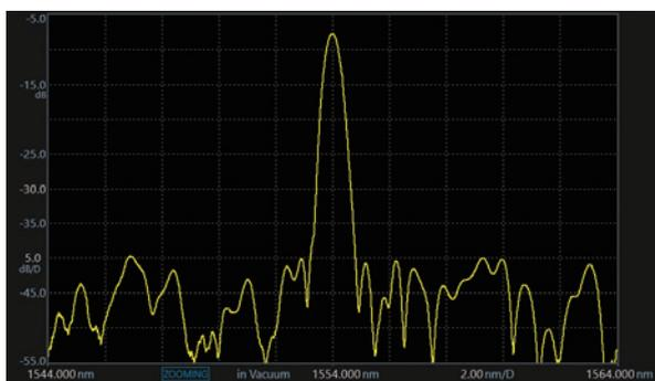
Transmission spectrum of optical filter
