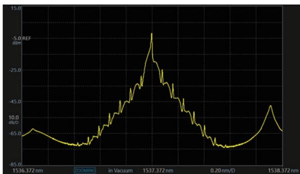
Modulated spectrum of 10G optical transceiver
